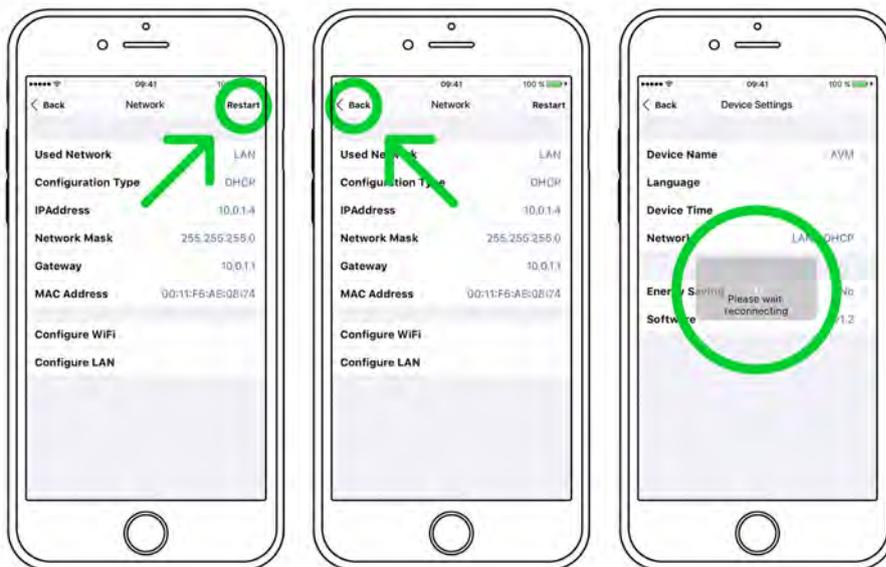
**CAUTION:** When switching from a wired ethernet connection (LAN) to a wireless WiFi connection or vice versa, a restart of the integrated streaming module of your SD 6.2 is always required. Please follow the above instructions to restart the device via the RC S App.
